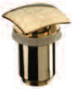
cod. A737 YG82 Squared automatic pop-up waste 1"1/4 with Click-Clack system with overflow
